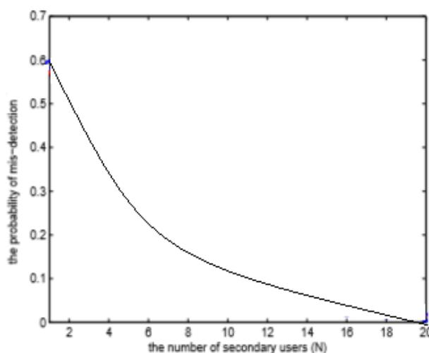
**Fig. 3** The average probability of mis-detection for various number of SUs
