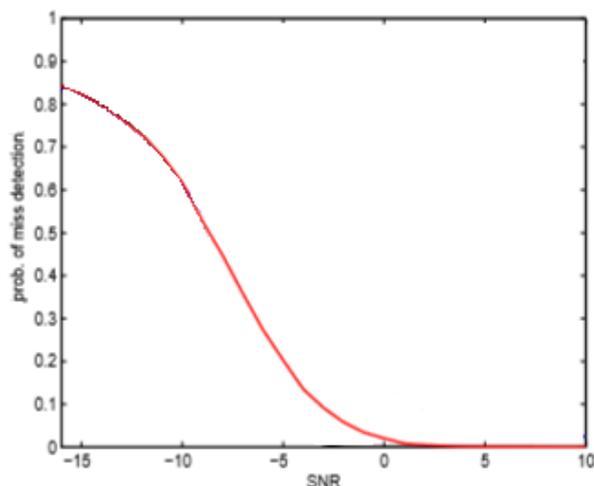
**Fig. 2** The average probability of mis-detection for various SNR
